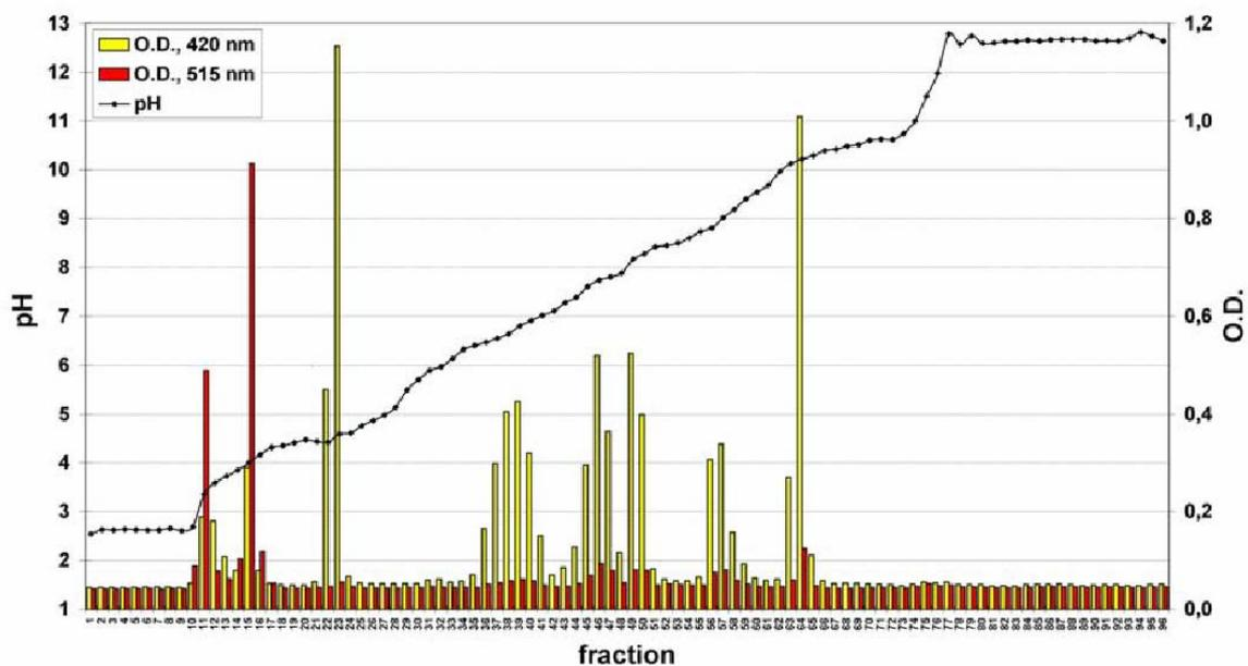
*pH-gradient in the separation chamber and the 96 fraction wells, respectively, as well as isoelectric focusing of six yellow and two red IEF-markers to demonstrate the performance of the Pro Team™ FFE instrument under the conditions used for the separation of membrane proteins.*
