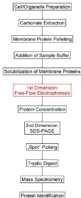
*Typical workflow for the FFE-based two-dimensional separation of membrane proteins*
