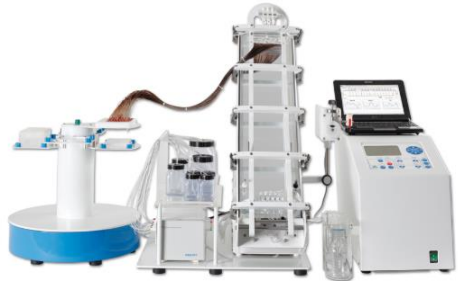
Figure 6: FFE unit with separation chamber, media pumps, power supply and collection robot. The cooling unit is not shown.
